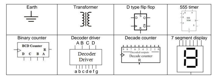
Circles can be put on S and R inputs for D types, and on CK and R inputs for counters (or bars over the letters) when inverted.
